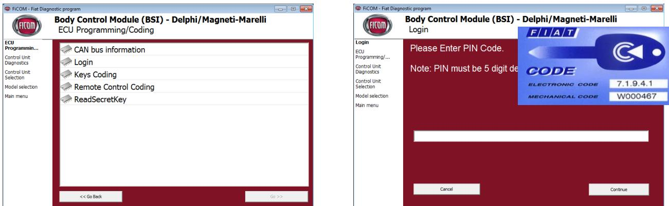
Coding transponders can be done by selecting the "Keys Coding" function. The procedure is as follows:
