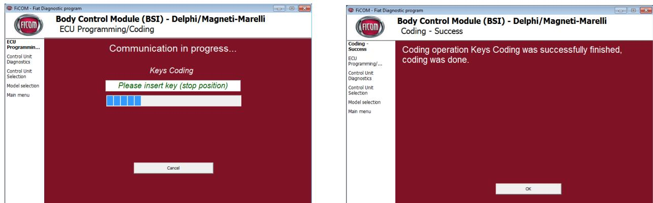
Previously deleted keys cannot be programmed again. Diagnostics can only add keys from system CODE2 and later (Megamos crypto + HiTag).
