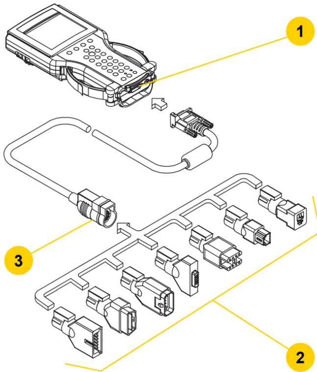
1. VCI cable connector (26-pin connector)
