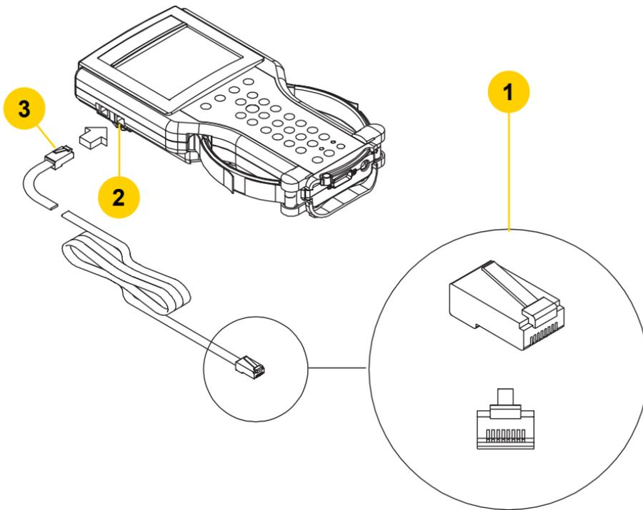
1. Detail of 8-pin RJ45 connector
